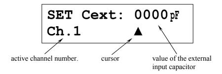
Use the keys **up** and **down** on the front panel to select the desired character. Hold **set** key down for longer than two seconds to move the cursor one step to the right. After the last position the cursor wraps around and starts at the first position again.
