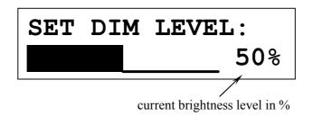
Additionally, the display shows the current brightness level in percent and by a bar of corresponding length:
