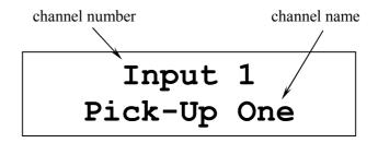
As soon as you enter the setup menu by pushing the **set** key, the display changes to show information related to the selected menu item. For further display details refer to the description of each menu item in section 'Setup menu' starting from page 25.
