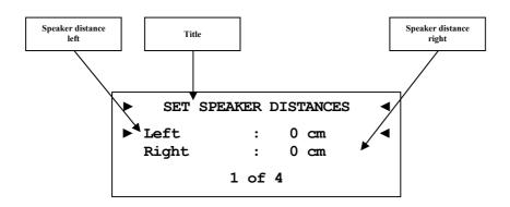
Use this menu to enter the distances from your speakers to your listening position. The distance ranges from 0 to 700 cm in steps of 5 cm. According to the entered distances, the DNP calculates the necessary delays of each channel to ensure that all signals from all speakers arrive at the same time at the listening position.
