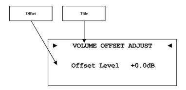
To offset differences between input devices, you can adjust the volume level for each channel in range from -9dB to +9dB.
