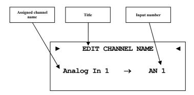
You can assign a fully user-definable name up to 12 characters in length to each of the seventeen input channels. The display shows the number of the currently selected input channel and the assigned channel name. The cursor marks the character you now may alter.
