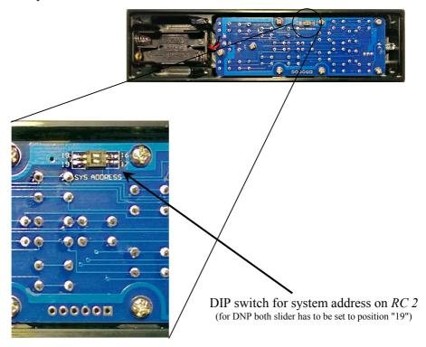
To configure the Audionet Metal Remote Control *RC 2* for controlling the DNP, put both sliders of the DIP switch labelled "SYS ADDRESS" in position "19".
