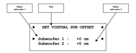
This option virtually moves the subwoofer relative to the listening position (= adjusting the phase of the subwoofer). Use **positive** values, if you want to **delay** the signal from the subwoofer relative to all other channels. Use **negative** values, if the signal from the subwoofer should arrive **earlier** than the signals from all other speakers.
