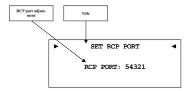
Enter the port number for communication between DNP and the software Audionet RCP or Android app aMM or iOS app iMM. If necessary, you may adjust the port number in a range of 50000 to 59999. The factory default value is 54321. Changing the default value will only be necessary if this port number is already used in your network. If necessary, ask your network administrator for support.
