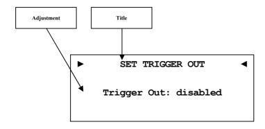
Use trigger output **TRIGGER** 5 to control (e.g. switch on/off) non Audionet devices. If you switch on the DNP from stand-by mode, the trigger output 5 provides a signal of 12 Volts DC.
