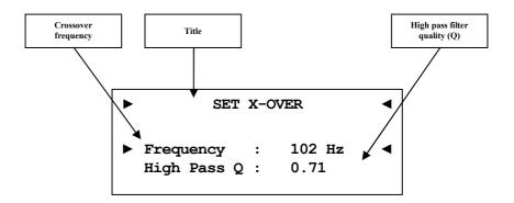
Now you have to adjust the cross over frequency for the speakers. The frequency defines the point of operation for the corresponding filters of your loudspeaker setup. Adjust the Q factor of the current high pass filter. The default setting is 0.71 and should only be altered by experts.
