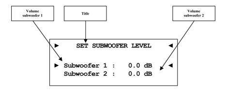
Adjust the differences in volume between mains channel Left / Right and subwoofer channel(s). If you setup your system to support two subwoofers, the DNP allows you to adjust both subwoofer volume offsets separately.
