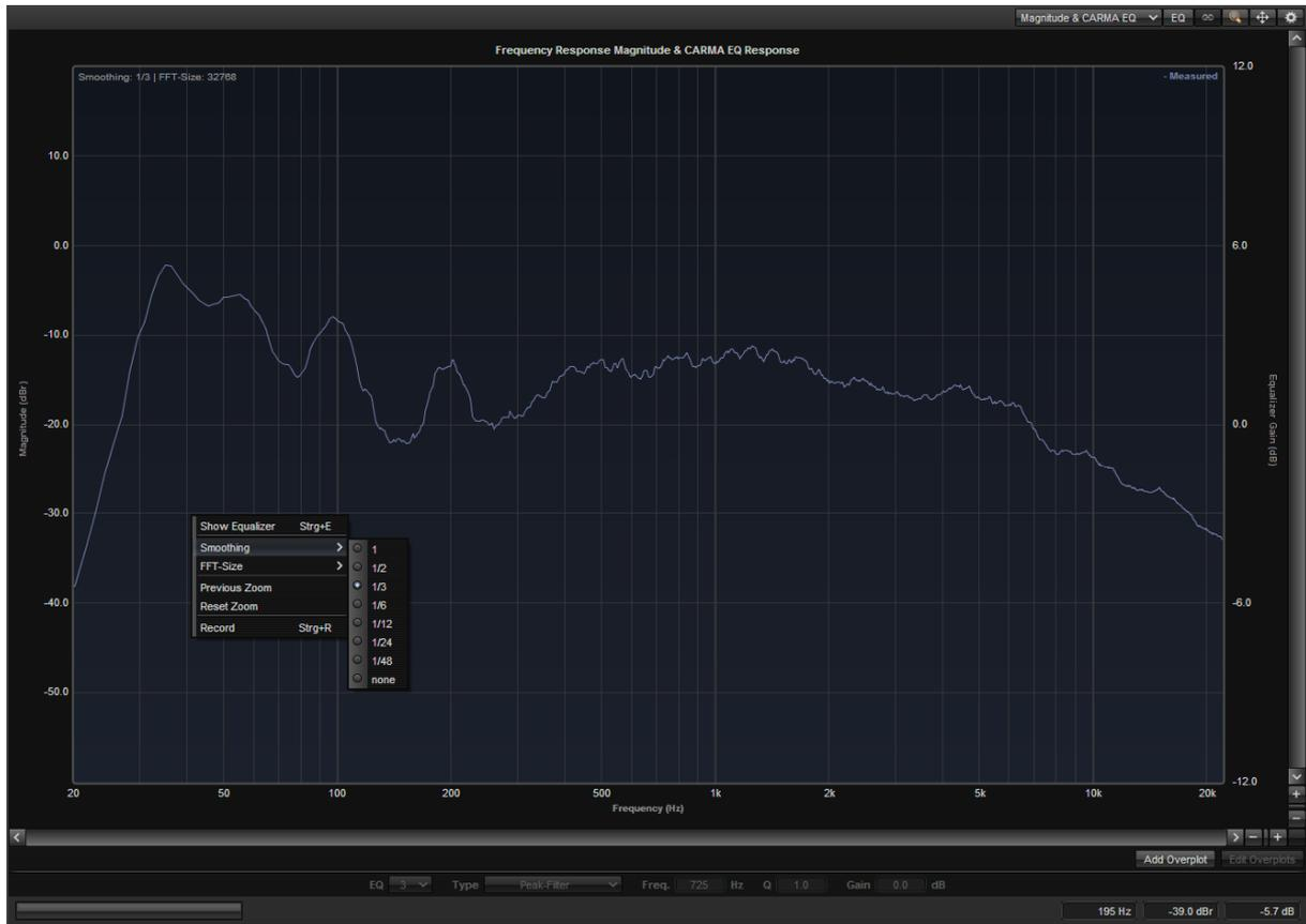
If the recording level is adjusted correctly the measured frequency response should be displayed considerably above the -30dB line. If not, you have to readjust the volume settings of your sound card and your amplifier. The screenshot below shows wrong measurements:
