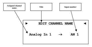
You can assign a fully user-definable name up to 12 characters in length to each of the eight input channels. The display shows the number of the currently selected input channel and the assigned channel name. The cursor marks the character you now may alter.
