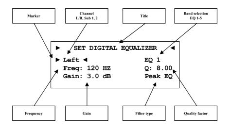
You can navigate through the menu of the digital EQ with the directional pad on your system remote control. With up/down keys you choose the parameter for adjustment, left/right changes the selected parameter. If you enter the digital equalizer menu item, the first selected parameter is **Left**. Here you select the speaker channel you want to adjust [**Left**, **Right**].
