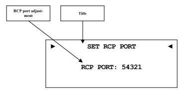
The communication port for software Audionet RCP and Android App aMM is set up here. This adjustment should only be done by professional users. Setup a value between 50000 to 59999. The default value has to be changed only if you have network communication problems. Ask your network administrator for support.
