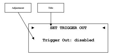
The trigger out connection could be used to remotely switch on/off non Audionet devices. By factory default the voltage is adjusted to 12V DC. If necessary the output voltage can be re-configured to 5V DC. Changing the voltage must be done by authorized personnel only. Ask your local dealer for support.
