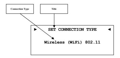
Wired EthernetFactory setting. Your DNC connects to a network<br/>via a connected network cable.Wireless (WiFi)Your DNC establishes a wireless connection via
