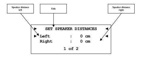
Use this menu to enter the distances from your speakers to your listening position. The distance ranges from 0 to 700 cm in steps of 5 cm. According to the entered distances, the DNC calculates the necessary delays of each channel to ensure that all signals from all speakers arrive at the same time at the listening position.
