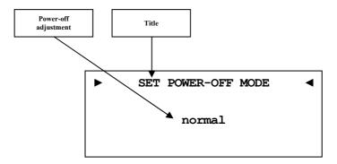
The DNC differentiates between two power-off modes. Firstly the **nor-mal** power-off mode and secondly the **Quick Start** mode.
