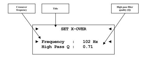
Now you have to adjust the cross over frequency for the speakers. The frequency defines the point of operation for the corresponding filters of your loudspeaker setup. Adjust the Q factor of the current high pass filter. The default setting is 0.71 and should only be altered by experts.
