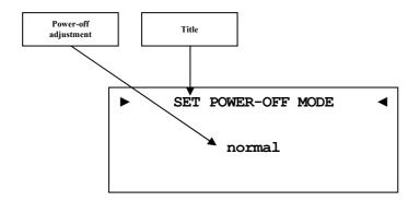
The DNA differentiates between two power-off modes. Firstly the **normal** power-off mode and secondly the **Quick Start** mode.
