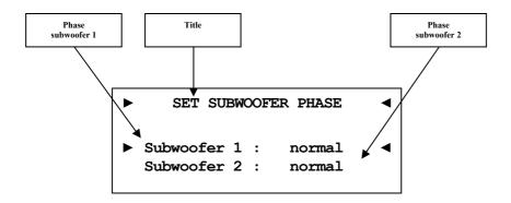
normal 0° phase shift inverted 180° phase shift
