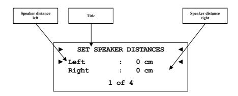
Use this menu to enter the distances from your speakers to your listening position. The distance ranges from 0 to 700 cm in steps of 5 cm. According to the entered distances, the DNA calculates the necessary delays of each channel to ensure that all signals from all speakers arrive at the same time at the listening position.
