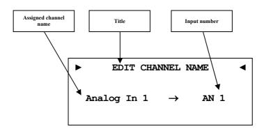
You can assign a fully user-definable name up to 12 characters in length to each of the thirteen input channels. The display shows the number of the currently selected input channel and the assigned channel name. The cursor marks the character you now may alter.
