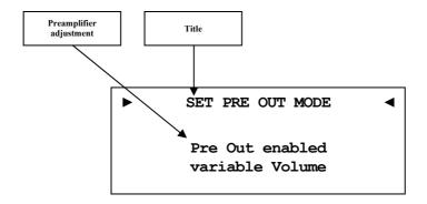
Pre Out enabled Preamplifier output is connected to variable Volume the volume control. Use this mode,
