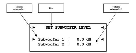
Use this adjustment to offset volume differences between subwoofer and main speakers. The subwoofer channels may be adjusted separately.
