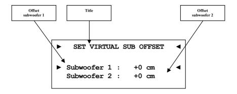
This option virtually moves the subwoofer relative to the listening position (= adjusting the phase of the subwoofer). Use **positive** values, if you want to **delay** the signal from the subwoofer relative to all other channels. Use **negative** values, if the signal from the subwoofer should arrive **ear-lier** than the signals from all other speakers.
