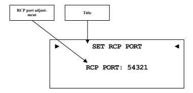
The communication port for software Audionet RCP and Android App aMM is set up here. This adjustment should only be done by professional users. Setup a value between 50000 to 59999. The default value has to be changed only if you have network communication problems. Ask your network administrator for support.
