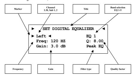
You can navigate through the menu of the digital EQ with the directional pad on your system remote control. With **up** / **down** keys you choose the parameter for adjustment, **left** / **right** changes the selected parameter. If you enter the digital equalizer menu item, the first selected parameter is **Left**. Here you select the speaker channel you want to adjust [**Left**, **Right**, **Subwoofer 1**, **Subwoofer 2**].
